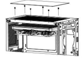
Put fan or water cooling on top panel from inner side and fix screws from outside
