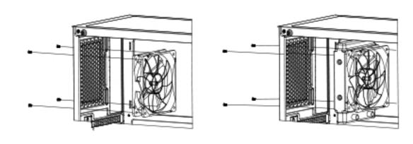
Put fan or water cooling on rear plate from inner side and fix screws from outside
