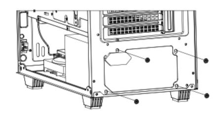
Lock 4pcs psu screws to fix psu
