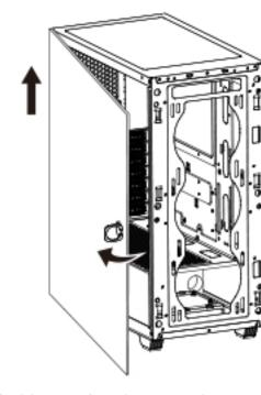
Open left side panel and remove the tempered glass side panel
