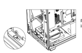
Put bracket on chassis after HDD installation, and lock 2pcs screws
