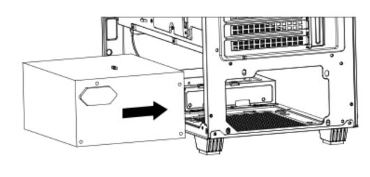
Put psu into chassis from left side
