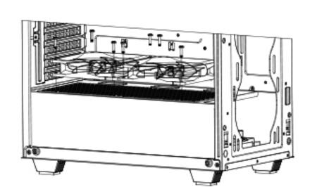
Put fan on upside of psu cover and fix screwss
