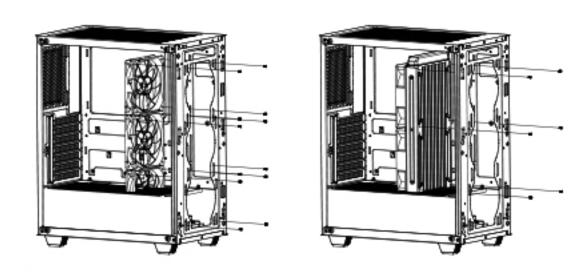
Put fan or water cooling on front plate from inner side and fix screws from outside
